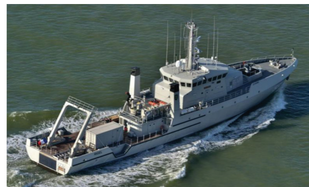
KRI RIGEL & KRI SPICA (Hydrographic ships) Owner : National navy of Indonesia Gearbox : MM W6400 + PTI 2 x Sets Engines : Electric + Diesel Equipment : Trolling mode + Shaft Brake Integrated
