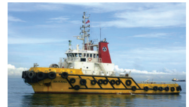
AN KANG (Towing Tug) Engines : 2 x GE 8V-228-900 rpm Gearboxes : 2 x MM W18000 NR Propellers : 2 x CPP MMS 640 Shipyard : SLS Korea
